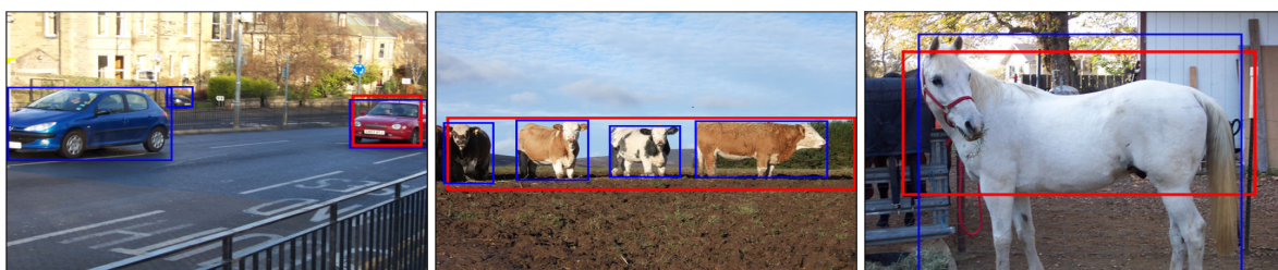
(b) Even with sufficiently many object features, localization errors occur: several objects are present, but we return only one per image (left), close or overlapping objects cause a single too big bounding box to be returned (center), small extended parts like legs can be missed (right).
