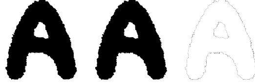
Figure 4. Area Difference: The size of a binarized letter (left) is increased slightly by raising the binarization threshold (center). The area of the additional pixels (right) typically is larger for inkjet printers than for laser and can be used for classification.
