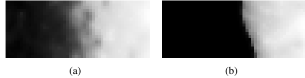
Figure 2. Enlarged contour region of a inkjet printed (a) and a laser printed character (b). The laser image shows a sharper black-to-white transition and fewer ink/toner droplets outside of the black contour.
