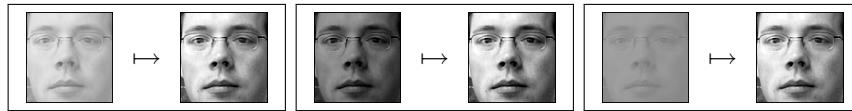
(a) Illumination invariance by brightness and contrast normalization. The right images are derived from the left by linearly transforming the grayvalues such that their minimum is 0 and their maximum is 1.
