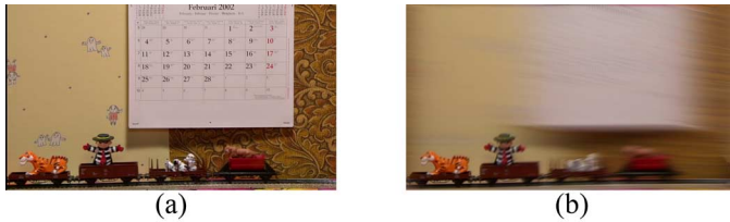
Fig. 9. Anisotropic filtering to selectively smoothen 2 + 1D video data. A strongly prolate anisotropic 3-D-Gaussian is aligned with the motion of the front of the toy train. The resulting filter acts as a motion aware blurring filter, only weakly smoothing the first two cars of the train, but strongly blurring the background and other objects which show different movement patterns. (a) Original frame #240. (b) Anisotropically filtered.
