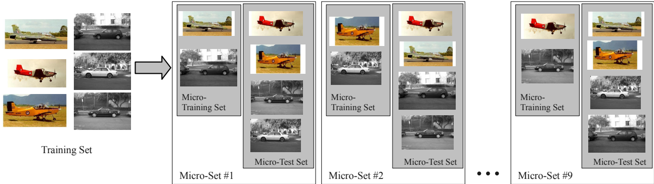
Figure 1. As shown above, a simple training set consisting of three example images for the two object classes, can be used to generate nine micro-sets. Each micro-set is one of the one-shot recognition problems that could be generated with the training set. The intermediate representation function, r(\mathbf{x}) , from Equation (5), is found by optimizing the probability of correct one-shot recognition across all of these sets.
