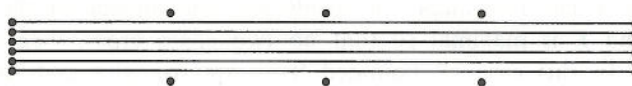
Fig. 3.1. An \Omega(mn) lower bound example on the number of vertices of a conforming Delaunay triangulation. In the example shown, m = 6 , k = 3 , and therefore n = 2m + 2k = 18 .
