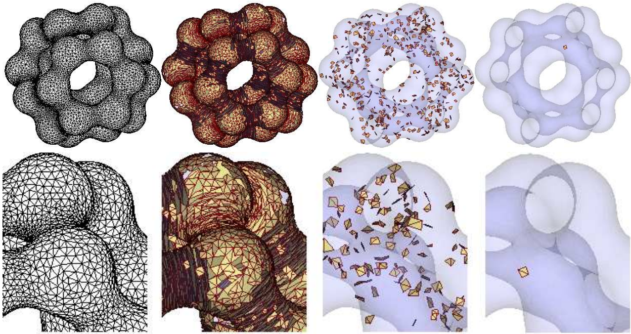
Figure 7: Permutahedron data. From left to right, surface mesh, initial Delaunay triangulation, Delaunay triangulation after refinement, and weighted Delaunay triangulation after exudation. The volume meshes are displayed by showing a transparent boundary surface together with opaque slivers. No other tetrahedra are shown.
